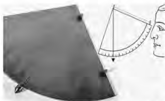
Figure 10-11: The quadrant is shaped from a quarter-circle. A weight hung on a string, from the center, creates a plumb line that crosses the lower graduated edge. The navigator sights the celestial body along the top edge, and the string crossing the lower arch shows the altitude, or angle, above the horizon where the measurement is being taken, which with the North Star gives you the latitude of your location.
