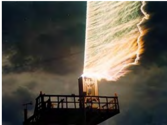
Artificial St Elmo's fire triggered by a tethered rocket.
