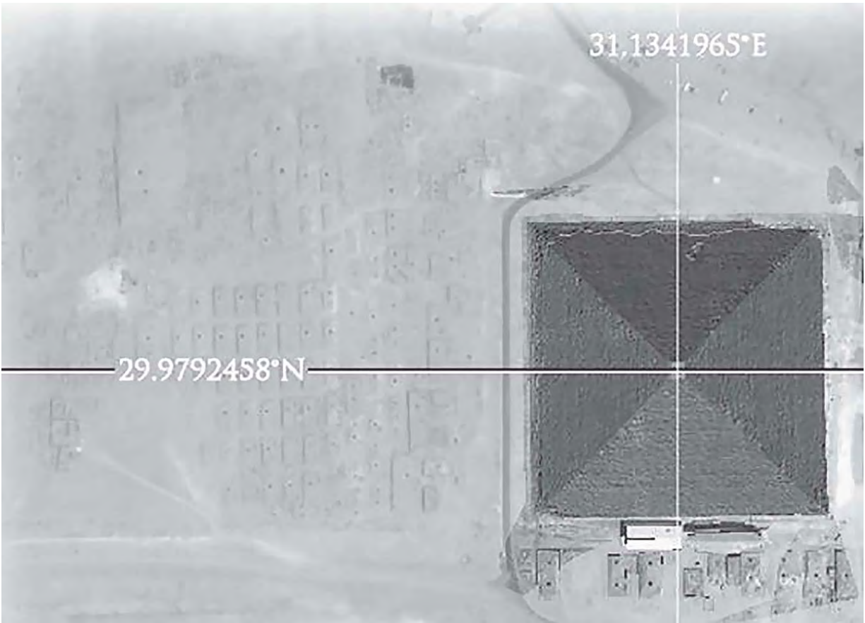
Fig. 11.38. The GPS-determined coordinates of the apex of the Great Pyramid
