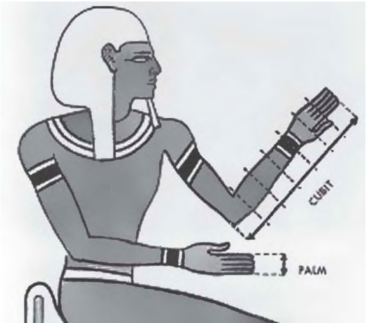
Fig. 11.22. The relationship between the palm and the cubit in ancient Egyptian measurement
