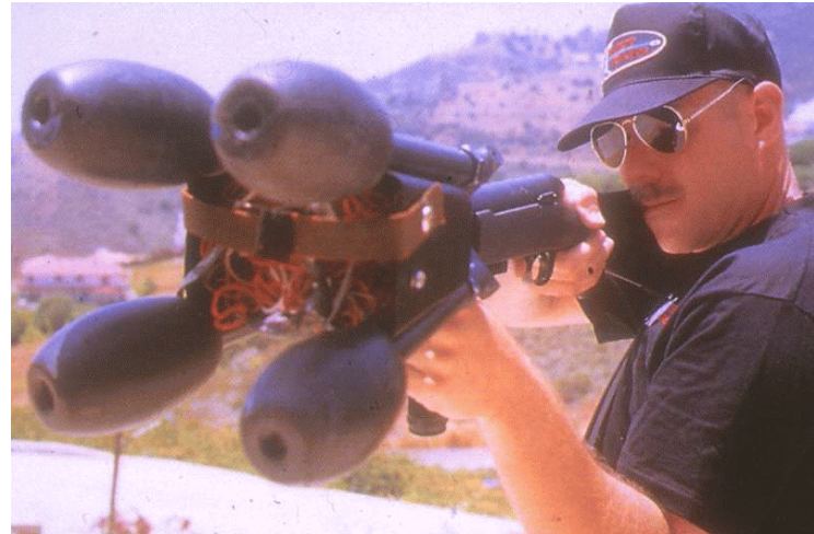
Fig. 12. Flight stabilised capture net.
