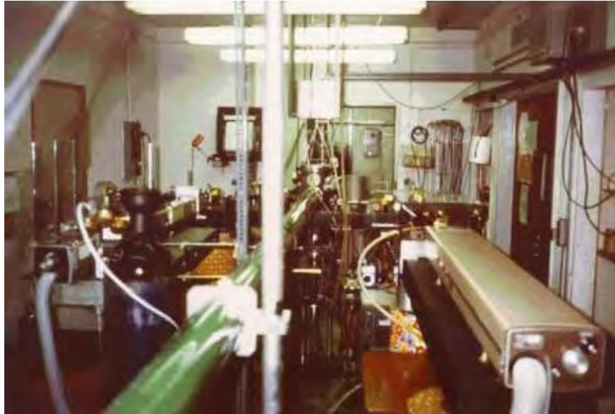
Figure 220: Aspect conducted his experiment in this lab at Orsay. The source of pairs of entangled photons consisted of several lasers, and a stream of atoms. Measurements were taken after they had travelled six meters in both directions from the source. (© GOA/LCFIO)
