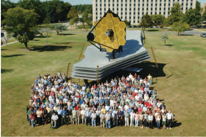
Plate 19 A full-scale model of the James Webb Space Telescope (JWST), the successor to the Hubble Space Telescope ( http://www.jwst.nasa.gov/ ; see Figure 10.2 and associated discussion for more information). JWST includes a primary mirror 6.5 m in diameter and offers instrument sensitivity across the IR wavelength range of 0.6 to 28\ \mu\text{m} , which will allow detection of the first generations of galaxies. The size of the Sun shield (the large flat screen in the image) is 22 in \times 10 m (72 ft \times 29 ft). The telescope will orbit 1.5 million km from Earth at the Lagrange L2 point. Courtesy of NASA/EPO.
