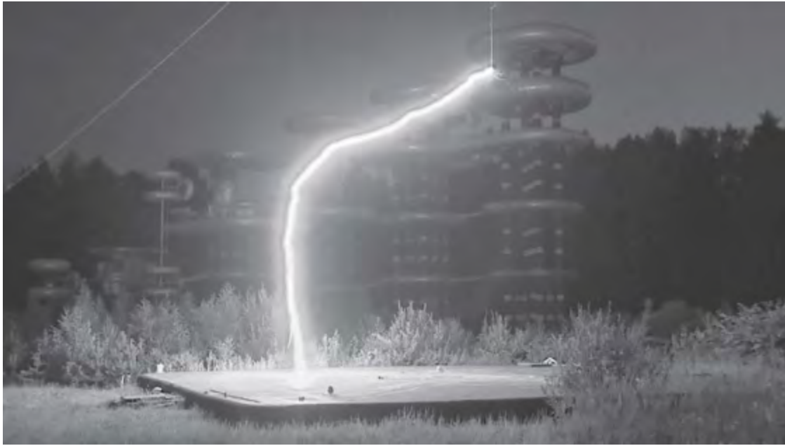
Fig. 1.7. The 6-megavolt Tesla Tower (a Marx generator, not a Tesla coil) at the High Voltage Research Center outside Moscow produces massive 200-meter volts of lightning and plasma arcs.
