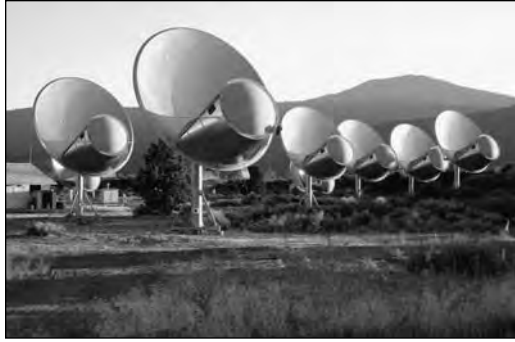
Figure 130. The Allen Telescope Array is planned to be a set of 350 six-meter radio dishes located in a lava-strewn valley north of San Francisco. Improvement in computers and signal processing means that large chunks of the radio spectrum can now be searched for signals that have no natural source. The array will provide a gain in speed on the sum of all previous SETI experiments by several orders of magnitude.
