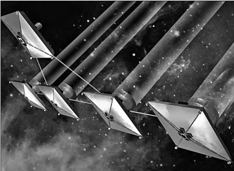
Figure 111. NASA's TPF interferometer is a set of four three- to-four-meter telescopes, either flying in precise formation or physically linked. Working at infrared wavelengths, it will be able to image terrestrial planets with a contrast of only one million to one. Spectra of the reflected planet light will reveal a different set of potential biomarkers. This mission therefore complements the coronagraph.
