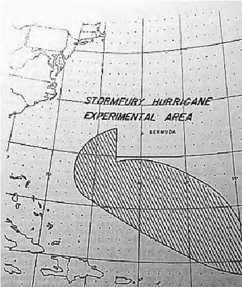
FIGURE 6.13. To reduce the risk of modified hurricanes striking land, Project Stormfury personnel could not seed any hurricanes unless they passed through this predetermined experimental area—a leftover precaution from Langmuir's 1947 modification attempt. From Project Stormfury, ESSA Fact Sheet, August 1966.
