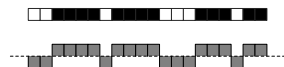
A sequence of discrete elements and a possible corresponding waveform for a sound.
