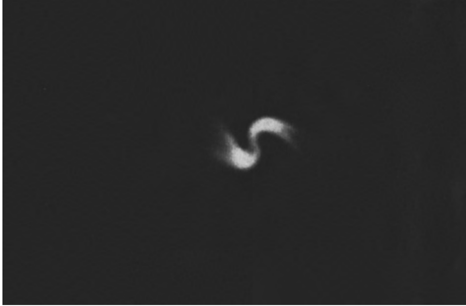
Figure 21. Bostick's photo, taken as a two-microsecond 'snapshot', showing what happened when he fired two plasmoids at each other. To his astonishment, they combined to form a 'barred spiral' shape resembling the well-known barred-spiral galaxies in space. As he wrote: 'Occasionally two plasmoids crashing head on break into fragments, but even these fragments seem to behave as entities. In other words, we appear to be dealing with bodies which have strong powers of self-organization and preservation.'
