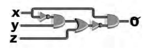
AND, OR, NOT, and COPY gates can be wired together to make logic circuits. A logic circuit can perform more complicated transformations of its input bits.
